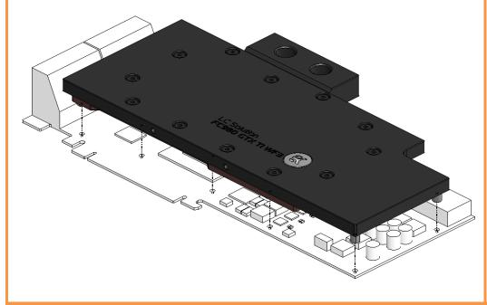
3. ATTACHING THE BLOCK TO THE GRAPHIC CARD. Use a Philips screwdriver screw with the enclosed M3x4 DIN 7985 screws. EKWB recommends users to start tightening the screws around the GPU core and continue outwards. <u>Always use</u> a plastic washer under each and every screw! If the washer is already present on the circuit board (usually around the four GPU core screw holes) there is no need for additional washer.
