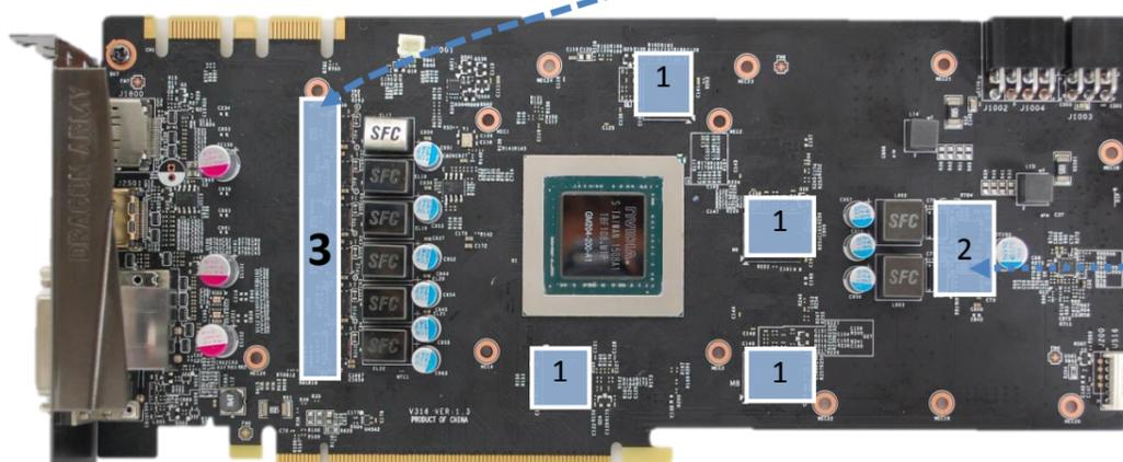
2. **PLACING THE BLOCK ON TO THE GRAPHICS CARD.** Carefully position the water block with preinstalled 2.5 mm standoffs on to the graphics card. During this process please make sure you align mounting holes on the PCB with holes on the water block (same applies for other tops). Also pay attention not to use too much force by pressing the block down to the PCB. Chip dies are prone to cracking.
