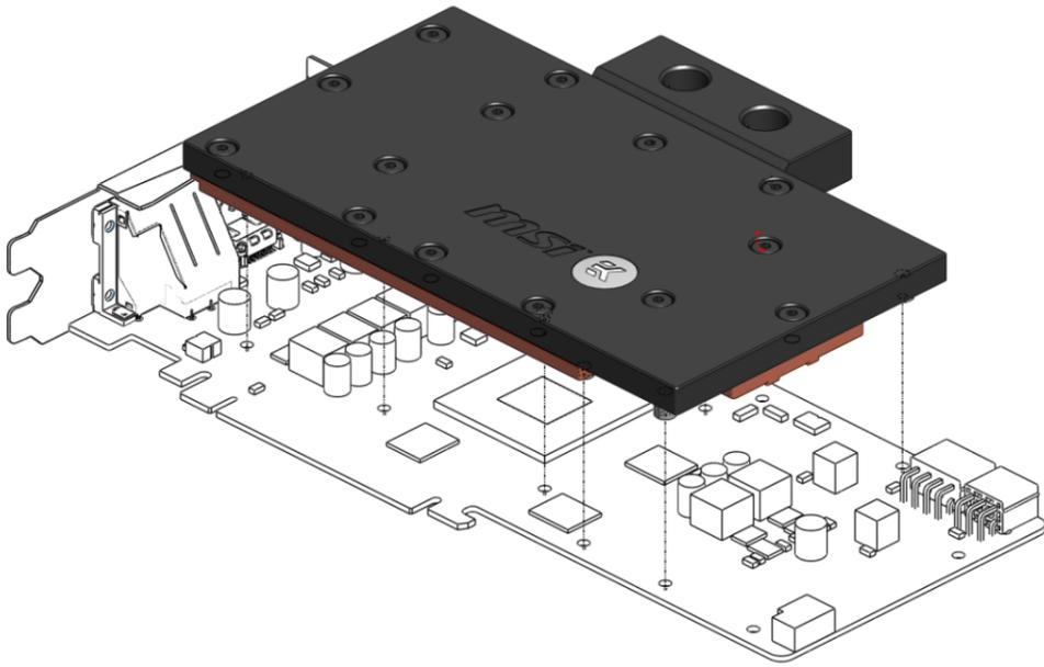
3. **ATTACHING THE BLOCK TO THE GRAPHIC CARD.** Use a Philips screwdriver with the enclosed M3x4 DIN 7985 screws. EKWB recommends users to start tightening the screws around the GPU core and continue outwards. Always use a plastic washer under each and every screw! If the washer is already present on the circuit board (usually around the four GPU core screw holes) there is no need for additional washer.
