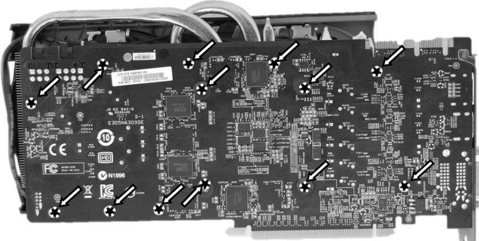
2. CLEANING THE PCB. Carefully detach the original stock cooler after removing **all** screws securing it to the board. Wipe off the remains (by using non-abrasive cloth or *q-tip*, as shown on sample photo) of the original thermal compound until the components and circuit board are completely clean. EKWB recommends the use of denatured alcohol for removing TIM leftovers.
