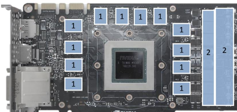
2. PLACING THE BLOCK ON TO THE GRAPHICS CARD. Carefully position the water block with preinstalled 2.5mm standoffs on to the graphics card. During this process please make sure you align mounting holes on the PCB with holes on the water block (same applies for other tops). Also pay attention not to use too much force by pressing the block down to the PCB. Chip dies are prone to cracking.
