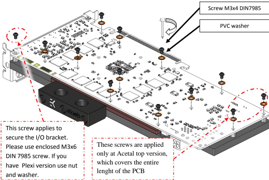
3. cont.: Secure the M3x6 DIN 7985 screw that holds the I/O bracket from the front side using M3 nut and PVC washer.
