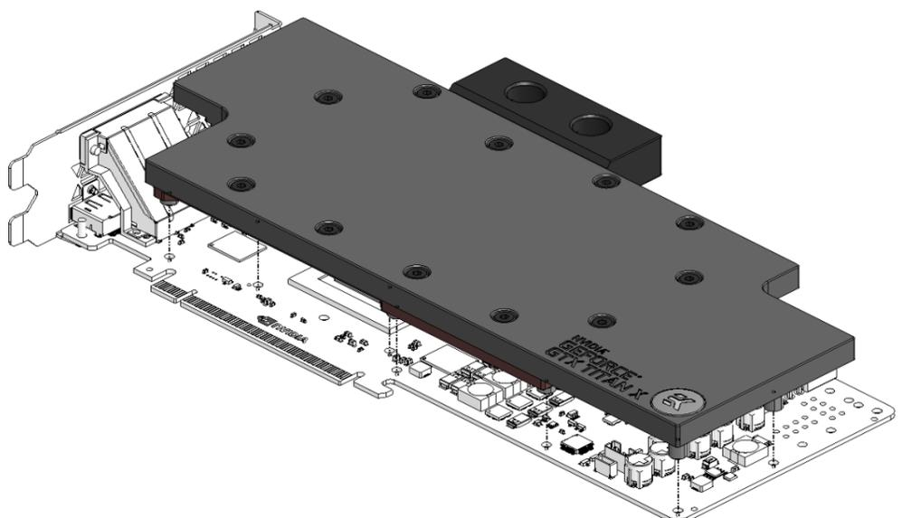
3. ATTACHING THE BLOCK TO THE GRAPHIC CARD. Use a Philips screwdriver with the enclosed M3x4 DIN 7985 screws. EKWB recommends users to start tightening the screws around the GPU core and continue outwards. To secure the I/O bracket please use enclosed M3x6 DIN 7985 screw.
