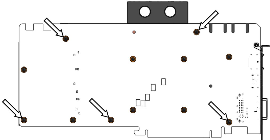
**STEP 3: APPLYING THE THERMAL PADS**
