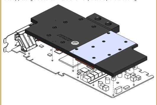
3. ATTACHING THE BLOCK TO THE GRAPHIC CARD. Use a Philips screwdriver screw with the enclosed M3x4 DIN 7985 screws. EKWB recommends users to start tightening the screws around the GPU core and continue outwards. <u>Always use</u> a plastic washer under each and every screw! If the washer is already present on the circuit board (usually around the four GPU core screw holes) there is no need for additional washer.
