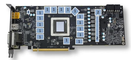
2. PLACING THE BLOCK ON TO THE GRAPHICS CARD. Carefully position the water block with preinstalled standoffs on to the graphics card. During this process please make sure you align mounting holes on the PCB with holes on the water block (same applies for other tops). Also pay attention not to use too much force by pressing the block down to the PCB. Chip dies are prone to cracking.
