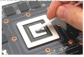
3. APPLYING THERMAL COMPOUND. Wipe off the remains (by using non–abrasive cloth or *q-tip*) of the original thermal compound until the components and circuit board are completely clean. Apply thermal compound: lightly coat *AMD* GPU chip with enclosed EK-TIM Ectotherm thermal grease. EKWB recommends to apply thermal grease in cross form for best performance (see sample picture).
