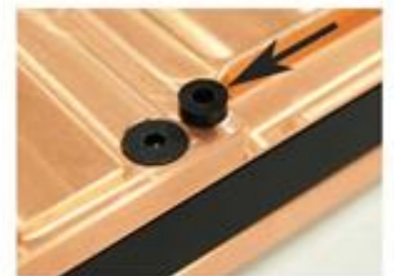
Then put the Stand-offs in center of the threads. Thermal grease helps that the stand-offs dont move while installing.
