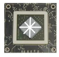
4. CUTTING THERMAL PADS. Your block comes with thermal pads, which have to be placed on chips (PLEASE REMOVE FOIL ON BOTH SIDES OF THERMAL PADS PRIOR TO INSTALLATION. WARNING: DIMENSION BELLOW ARE SCALED.) All thermal pads are **1mm** thick. Thermal pads #1 need to be cut to 4 pieces for RAM modules.
