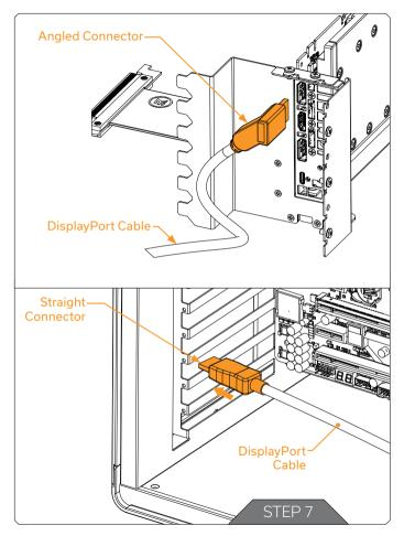
Before you mount the GPU Holder in your PC, connect the angled connector of the enclosed DisplayPort cable to the GPU, then pull the cable's straight connector through the horizontal bars (where you previously removed the PCIE brackets).
