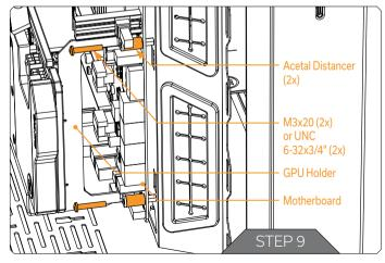
Use three or more screws to attach the GPU Holder to the left side of the PC case.
