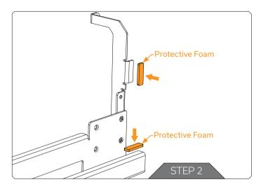
Stick two protective adhesive foams, as indicated in the diagram. The »2mm protective foam« should be enough for the protection of your GPU during installation. In some cases, you may use the »5mm protective foam« (also enclosed in the package) for the extra support of your GPU.
