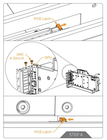
Before you mount the GPU, make sure the PCIE latch is not closed – it must be pushed to the right side.
