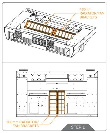
To install the radiators, all of the fan mounting brackets must be removed.
