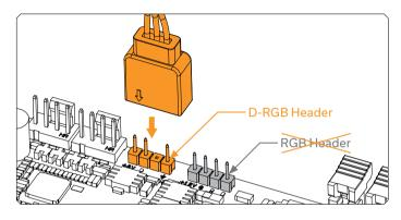
Plug the 3-pin connector of the distribution plate D-RGB LED light to the D-RGB header on the motherboard. The LEDs will work if the pin layout on the header is as follows: **+5V, Data, Empty, Ground.**
