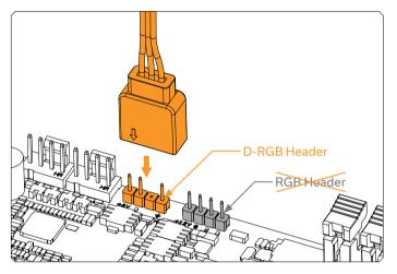
Connect the 3-pin D-RGB LED connector from your Flow Indicator to the D-RGB header on your motherboard or controller. The lights will work if the pin layout on the header is as follows: **+5V, Data, Empty, Ground**.
