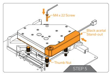
Push the black acetal stand-out back to its original position and screw back the  $M4 \times 22$  screw that was removed at Step 2.
