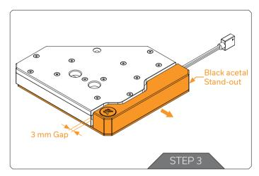
Slide the black acetal stand-out with stainless steel fixation plate away from the plexi components until it stops (approximately at 3mm).
