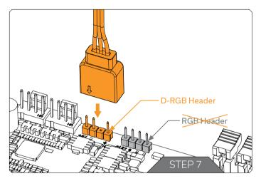
Plug the 4-pin D-RGB connector from the bridge block in a D-RGB header on your motherboard or controller. The LED strip will only work if the pin layout on the header is as follows: **+5V**, Digital, Empty, Ground.
