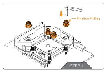
Install your EK-Quantum Velocity or Velocity Strike CPU water block in the illustrated orientation and place the motherboard on a secure flat surface. Using the enclosed 8mm Allen key, install all four (4) fixation fittings to the pre-installed VRM block and CPU block.
