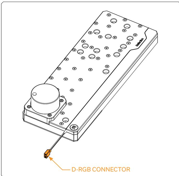
Plug the 3-pin connector of the distribution plate D-RGB LED light to the D-RGB HEADER on the motherboard. The LED will work if the pin layout on the header is as follows: +5V, Digital, Empty, Ground.
