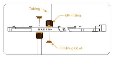
Screw in two male G1/4 threaded fittings. Attach the liquid cooling tubes and connect the water-block(s) into the cooling loop. **EKWB recommends using EK- fittings with the EK-Vector series water blocks.**
