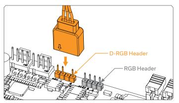
Plug the 3-pin connector from Water Block strip to the motherboard.
