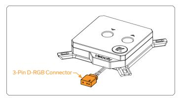
Plug the 3-pin connector from the water block's D-RGB LED light in the D-RGB HEADER on the motherboard. The LED will work if the pin layout on the header is as follows: +5V, Digital.
