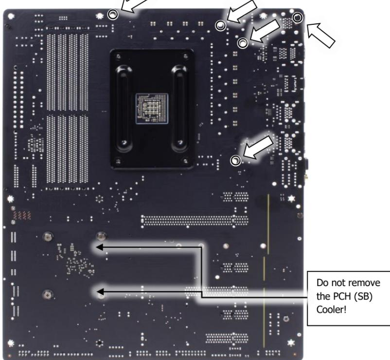
**Removing of the original plastic hold-down clamps and the factory backplate:** Using Philips-head screwdriver remove the four UNC 6-32 screws securing the original plastic hold-down clamps around the socket as shown on the sketch. Remove the original AMD® backplate and the hold-down clamps and store them away.
