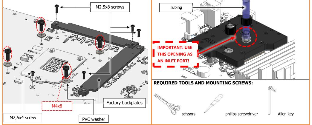
For the EK-FB ASUS M8E Monoblock series water block to operate properly the G1/4 port nearest to the right edge of the water block **MUST BE USED AS THE INLET PORT**. EK recommends the use of EK-ACF fittings. When using fittings other than EK-ACF series please use hose clamps or appropriate substitute to secure the tubing to the barb. The use of biocide containing and corrosion inhibiting coolant is always recommended for any liquid cooling system.
