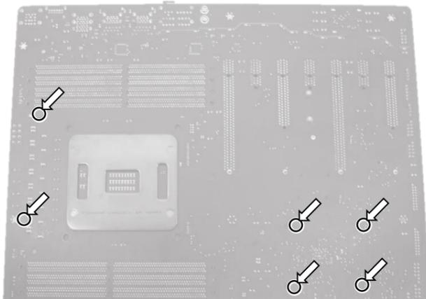
2. **CLEANING THE PCB.** Carefully detach the original stock cooler after removing **all** screws securing it to the board. Wipe off the remains (by using non-abrasive cloth or *qtip*, as shown on sample photo) of the original thermal compound until the components and circuit board are completely clean. EKWB recommends the use of denatured alcohol for removing TIM leftovers.
