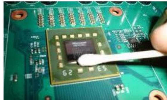
3. **APPLYING THERMAL COMPOUND.** Apply thermal compound: lightly coat the *Intel X99 PCH (SB)* with electrically non-conductive thermal grease - for example Arctic Cooling MX-2™, MX-4™ or GELID GC-Extreme™. EKWB recommends to apply the thermal grease in cross form for the best performance (see sample picture).
