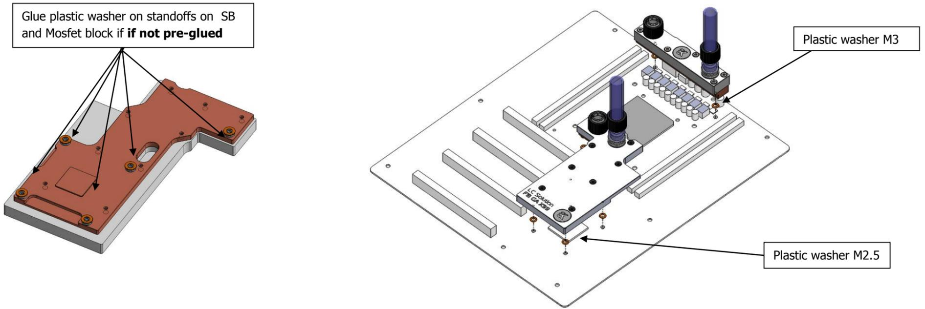
**STEP 4: ATTACHING THE BLOCK TO THE MOTHERBOARD**
