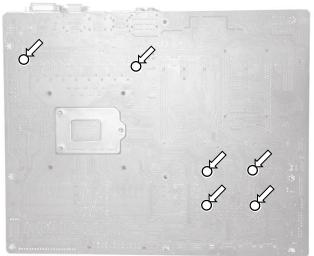
2. CLEANING THE PCB. Carefully detach the original stock cooler after removing **all** screws securing it to the board. Wipe off the remains (by using non-abrasive cloth or *qtip*, as shown on sample photo) of the original thermal compound until the components and circuit board are completely clean. EKWB recommends the use of denatured alcohol for removing TIM leftovers.
