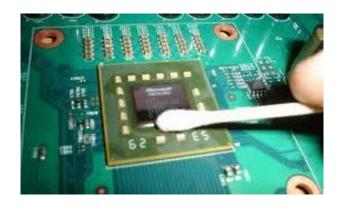
3. APPLYING THERMAL COMPOUND. Apply thermal compound: lightly coat the *Intel Z97 PCH* (SB) with <u>electrically non-conductive</u> thermal grease - for example Arctic Cooling MX-2  $^{\text{TM}}$ , MX-4  $^{\text{TM}}$  or GELID GC-Extreme  $^{\text{TM}}$ . EKWB recommends to apply the thermal grease in cross form for the best performance (see sample picture).
