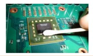
3. APPLYING THERMAL COMPOUND. Apply thermal compound: lightly coat the AMD 4. CUTTING THERMAL PADS. Your block comes with two thermal pads which needs to 990FX (NB) with electrically non-conductive thermal grease - for example Arctic Cooling MX-2 ™, MX-4 ™ or GELID GC-Extreme ™. EKWB recommends to apply thermal grease in cross form for best performance (see sample picture).
