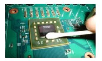
3. APPLYING THERMAL COMPOUND. Apply thermal compound: lightly coat the *Intel C606* (PCH) as well as PCIe PLX PEX8784 bridge chip with <u>electrically non-conductive</u> thermal grease - for example Arctic Cooling MX-2 <sup>TM</sup> or MX-4 <sup>TM</sup>. EKWB recommends to apply thermal grease in cross form for best performance (see sample picture).
