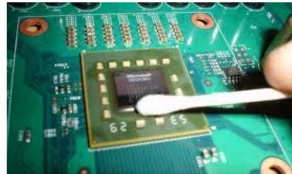
3. APPLYING THERMAL COMPOUND. Apply thermal compound: lightly coat the *Intel X79 PCH (SB)* with electrically non-conductive thermal grease - for example Arctic Cooling MX-2™ or MX-4™. EKWB recommends to apply thermal grease in cross form for best performance (see sample picture).
