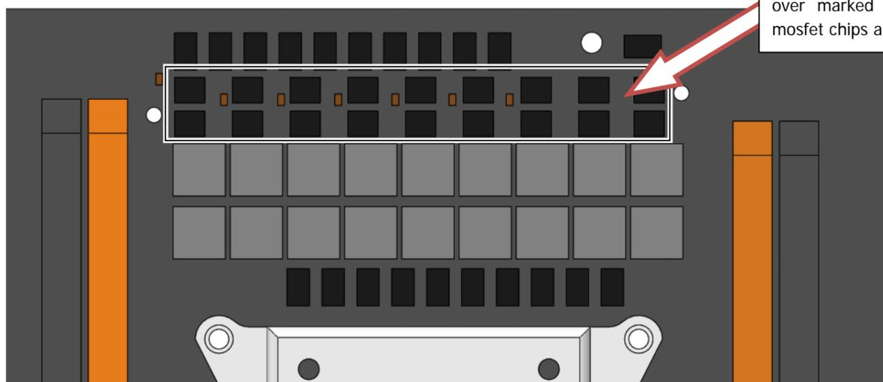
Place 0.5mm thermal pad in large strip over marked area and make sure all mosfet chips are covered.
