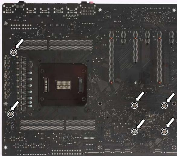
2. CLEANING THE PCB. Carefully detach the original stock cooler after removing all screws securing it to the board. Wipe off the remains (by using non-abrasive cloth or *qtip*, as shown on sample photo) of the original thermal compound until the components and circuit board are completely clean. EKWB recommends the use of denatured alcohol for removing TIM leftovers.
