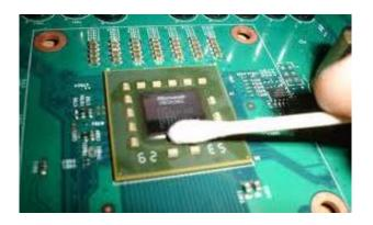
3. APPLYING THERMAL COMPOUND. Apply thermal compound: lightly coat the *Intel X79 PCH* (SB) with <u>electrically non-conductive</u> thermal grease - for example Arctic Cooling MX-2  $^{\text{TM}}$  or MX-4  $^{\text{TM}}$ . EKWB recommends to apply thermal grease in cross form for best performance (see sample picture).
