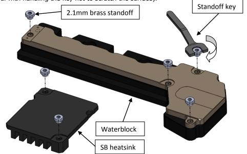
motherboard or vice versa. Make sure that mounting holes are aligned. Repeat the same with SB heatsink.
