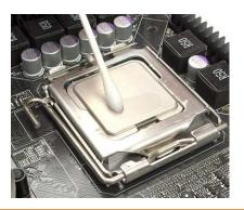
3. APPLYING THERMAL COMPOUND. Apply thermal compound: lightly coat the *AMD 990FX* (NB) as well as *SB950* (SB) chip with <u>electrically non-conductive</u> thermal grease - for example Arctic Cooling MX-2  $^{\text{TM}}$  or MX-4  $^{\text{TM}}$ . EKWB recommends to apply thermal grease in cross form for best performance (see sample picture).
