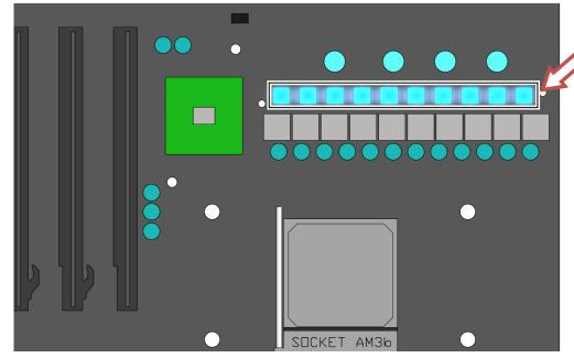
Place thermal pads in marked area and make sure all mosfet chips are covered.
