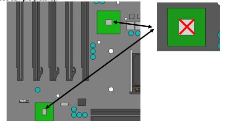
4. CUTTING THERMAL PADS. Your block comes with one precut thermal pad (90x15x1mm) which needs to be trimmed a bit in order to fit the voltage regulation area (VRM/MOSFET) on the motherboard's circuit board. WARNING: DIMENSIONS ON PICTURES BELLOW ARE SCALED!
