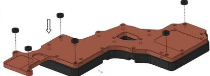
2. PLACING BLOCK OVER GPU. Place the motherboard on the inverted water blocks or vice versa and attach them with enclosed screws as shown. Make sure that mounting holes are aligned.
