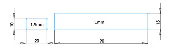
5. PLACING THERMAL PADS ON MOTHERBOARD. Place thermal pads you cut on PCB as shown on picture bellow. (PLEASE REMOVE FOIL OF THERMAL PADS ON BOTH SIDES PRIOR TO INSTALLATION.)
