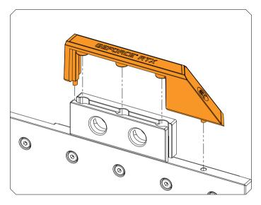
Take the pre-assembled D-RGB Terminal Cover from the box and attach it to the FC Terminal.
