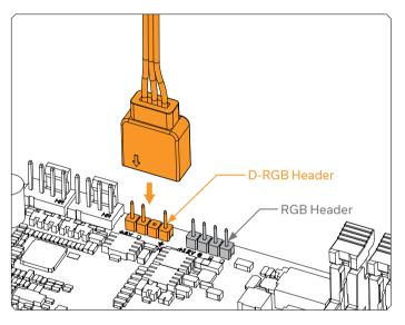
Plug the 3-pin connector from the water block's D-RGB LED light in the D-RGB HEADER on the motherboard. The LED will work if the pin layout on the header is as follows: +5V, Digital.
