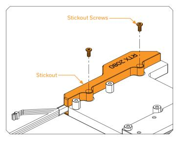
Remove the Stickout from the water block and store the screws for later use.
