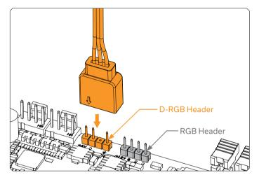
Plug the 3-pin connector from Water block's D-RGB LED light to the DRGB HEADER on the motherboard. The LED will work if the pin layout on the header is as follows: +5V, Digital, empty, Ground.
