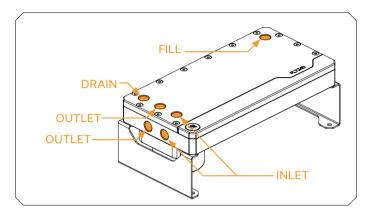
EK-Quantum Kinetic FLT has two inlet and two outlet ports, one of each must be used! All 4 unused ports should be blocked using G1/4 plugs.
