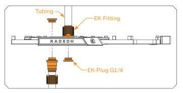
Screw in two male G1/4 threaded fittings. Attach the liquid cooling tubes and connect the water-block(s) into the cooling loop. **EKWB recommends using EK- fittings with the EK-Vector series water blocks.** If you are using barb fittings please add hose clamps or an appropriate substitute to ensure that the tubes are firmly secured. You can configure any port as an inlet or outlet. Do not forget to plug all remaining ports with the enclosed EK-Plug G1/4 or equivalents.
