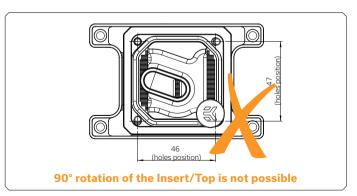
For AM4/AM5 versions it is not recommended to rotate the Insert relative to the CPU socket due to its asymmetrical design.
