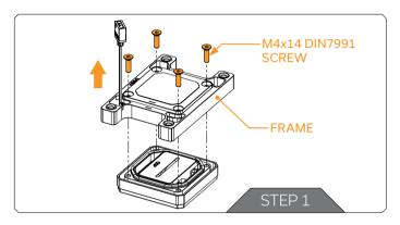
It is possible to exchange the Accent on any Magnitude CPU Water Block for an Accent with a different color or material finish. A translucent D-RGB Accent can also be used to add lighting to any version of Magnitude with an opaque Top.
