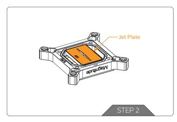
Choose the appropriate Jet Plate according to the table below, ensure that it is correctly aligned in the Insert and the O-Rings remain in position.
