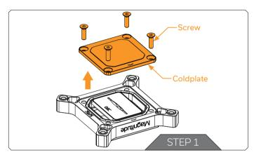
Original Magnitude Coldplates have a subtle curvature to achieve the best possible contact with the IHS of standard CPU's. If you choose to replace or modify the IHS it is also possible to replace the Coldplate of your Magnitude with a Flat version. To install the Flat Coldplate or to re-install your original Curved Coldplate follow these instructions:
