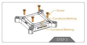
Put the desired Coldplate in place paying attention to the orientation, failure to do so will prevent installation of the Screws. The curvature marking should be on the same side as the curvature marking of the Frame. Lastly screw in the four Screws, do not use excessive force!
