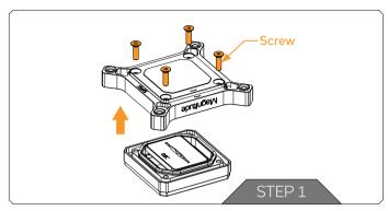
Unscrew the four Screws from the bottom of the CPU Water Block in an anticlockwise direction, then remove the Frame and Coldplate. A 2.5mm Allen (hex) key is supplied for this. If an LED Strip is already installed and you do not wish to change where the cable exits then the Frame does not need to be removed from the cable.
