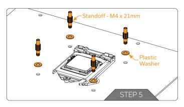
Loosely install all four Standoffs and Plastic Washers before proceeding to tighten them completely. It is mandatory for 115X and AM4 to install the Plastic Washers as they prevent damage to the motherboard PCB. Using pliers or similar tools is not recommended.
