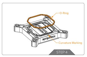
Put the Frame into place and then refit the O-Ring between the Frame and Top. Pay attention to the orientation of the Frame, failure to do so will prevent installation of the Screws. The curvature marking should be in line with either end of the Jet Plate opening as illustrated.
