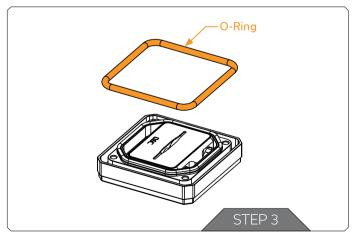
**STEP 3 (WITHOUT LED STRIP)**If applicable refit the O-Ring between the Top and Accent. This is not required for operation of the block but ensures the Accent is tightly fitted without an LED Strip.
