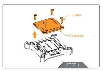
All Magnitude CPU Water Blocks are supplied with an additional Jet Plate that is 0.1mm thicker than the default Jet Plate. If the Coldplate touches the edges of the IHS and prevents optimal contact in the center then it is recommended to install the thicker Jet Plate.
