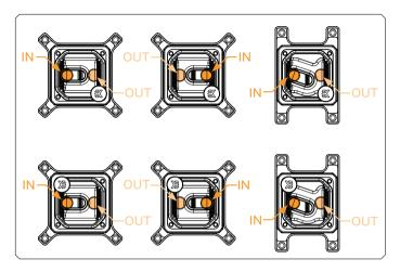
Magnitude 115X and 20XX CPU Water Blocks can be assembled with each part in multiple orientations to deliver exactly the same thermal and hydraulic performance when the flow direction or branding must be reversed. For AM4 versions it is not recommended to rotate the Insert relative to the CPU socket due to its asymmetrical design. The following orientations will deliver optimal performance:
