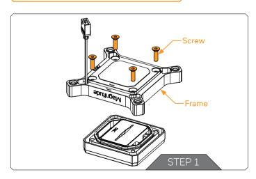
It is possible to exchange the Accent on any Magnitude CPU Water Block for an Accent with a different color or material finish. A translucent D-RGB Accent can also be used to add lighting to any version of Magnitude with an opaque Top.
