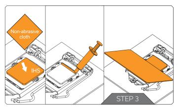
Wipe the IHS clean using a non-abrasive cloth or Q-tip as shown in the illustration. Once clean apply a line of Thermal Compound on one edge of the IHS and use a credit card or similar to spread it evenly.
