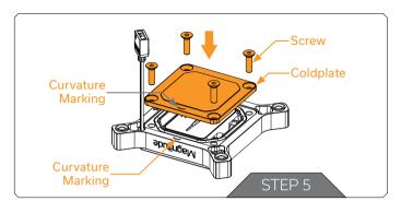
Replace the Coldplate, pay attention to the orientation, failure to do so will prevent installation of the Screws. The curvature marking should be on the same side as the curvature marking of the Frame. Lastly screw in the four Screws, do not use excessive force!
