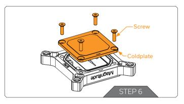
Replace the Coldplate paying attention to the orientation, failure to do so will prevent installation of the Screws. The curvature marking should be on the same side as the curvature marking of the Frame. Lastly screw in the four Screws, do not use excessive force!
