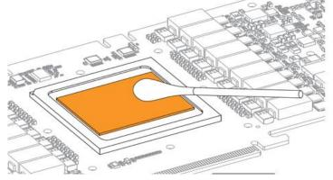
3. CUTTING THERMAL PADS: Your block comes with thermal pads, some of which are already precut. Others have to be cut to smaller chunks in order to cover all the VRM components such as MOSFETs and drivers. PLEASE REMOVE THE PROTECTIVE FOIL FROM BOTH SIDES OF THE THERMAL PADS PRIOR TO INSTALLATION. BAG CONTENT: Bag content is universal for all water blocks, you may not need all screws.
