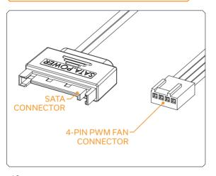
The EK-D5 PWM pump has two connectors.
