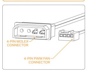
The EK-D5 PWM pump has two connectors.
