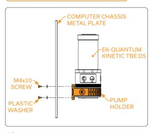
By default the EK-Quantum Kinetic TBE D5 ships with a pump holder that can be installed directly to the computer chassis. If there are no appropriate mounting holes available: user may need to drill 4 (four)  $\Phi$ 5 mm holes through the metal chassis using an electric power drill. Included is a sticker which can be used to mark the hole centers accurately.
