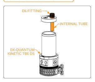
The internal tube, which is enclosed in a mounting kit, can be used for fluid intake into the reservoir. Make sure that the sealing gasket on the internal tube is placed correctly.
