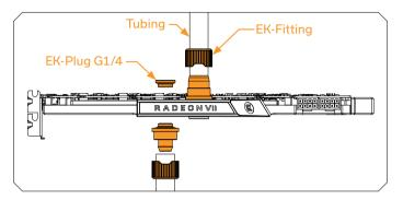
Screw in two male G1/4 threaded fittings. Attach the liquid cooling tubes and connect the water-block(s) into the cooling loop. **EKWB** recommends using **EK-STC or EK-HTC fittings with the EK-Vector series water blocks.** Tlf you are using barb fittings please add hose clamps or an appropriate substitute to ensure that the tubes are firmly secured.
