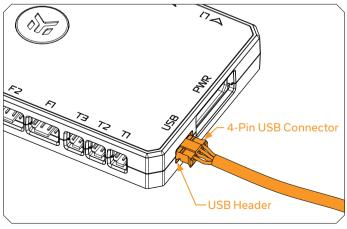
The other end of the USB cable should be plugged into the Connects USB port.
