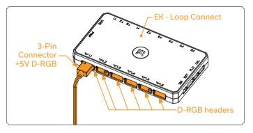
There are 6 Lighting headers marked with L1-L6, these headers are compatible only with 5V D-RGB products and LED strips! Make sure that the arrows are aligned.
