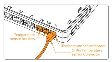
Optionally up to 3 temparature sensors may be installed to the headers marked T1-T3.
