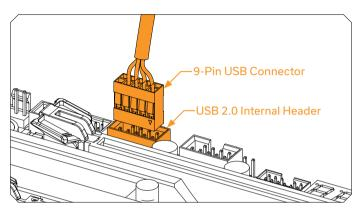
EK-Loop Connect must be linked to the motherboard using the supplied Internal USB 2.0 cable. Connect the 9-pin end to a USB2.0 header on the motherboard, pay attention to the orientaiton of the missing pin.
