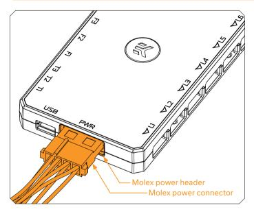
Finally plug in the Molex power connector to the PWR port using either a Molex connector directly from your PSU or the supplied 2x SATA Power adapter.
