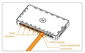
The controller is compatible with 4-pin PWM Fans, 3-pin Fans may be used however it will not be possible to adjust the speed. Insert the 4-pin Fan connectors as shown below to the 6 Fan headers marked F1-F6
