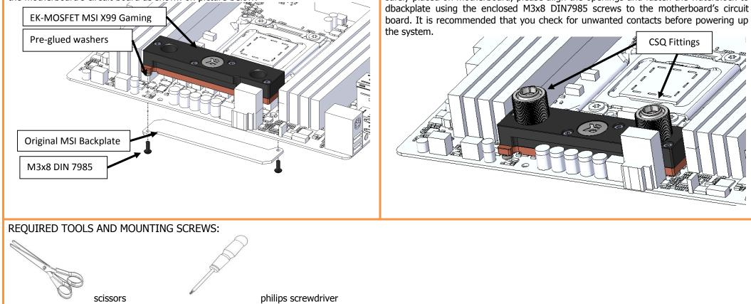
ATTACHING WATERBLOCK/BACKPLATE ON MOTHERBOARD. When waterblock is safely placed on motherboard, please align the openings and fasten the waterblock to
