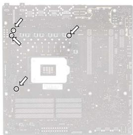
2. CLEANING THE PCB. Carefully detach the original stock cooler after removing **all** screws securing it to the board. Wipe off the remains (by using non–abrasive cloth or *q-tip*, as shown on sample photo) of the original thermal compound until the components and circuit board are completely clean. EKWB recommends the use of denatured alcohol for removing TIM leftovers.
