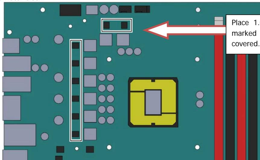
Place 1.0mm thick thermal pads in larger strips over marked area and make sure all mosfet chips are covered.
