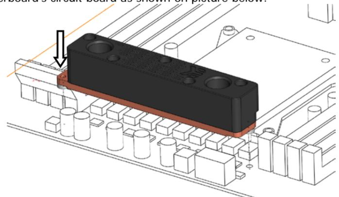
3. ATTACHING WATERBLOCK/BACKPLATE ON MOTHERBOARD. When waterblock is safely placed on motherboard, please align the openings and fasten the waterblock to enclosed backplate using the enclosed M3x10 DIN7985 screws and plastic washers to the motherboard's circuit board. It is recommended that you check for unwanted contacts before powering up the system.
