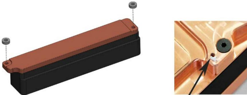
2. PLACING WATERBLOCK ON MOTHERBOARD. Place waterblock on VRM section of the motherboard's circuit board as shown on picture below:
