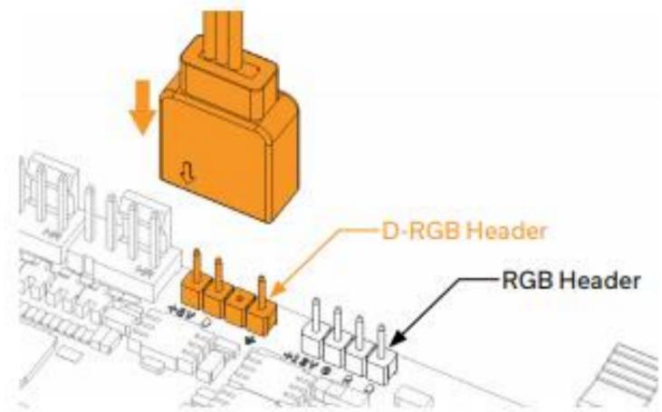
**STEP 4: ATTACHING BLOCK ON TO THE MOTHERBOARD**
