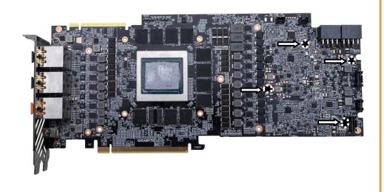
2. APPLYING THERMAL COMPOUND: Wipe off the remains (by using non-abrasive cloth or q-tip) of the
