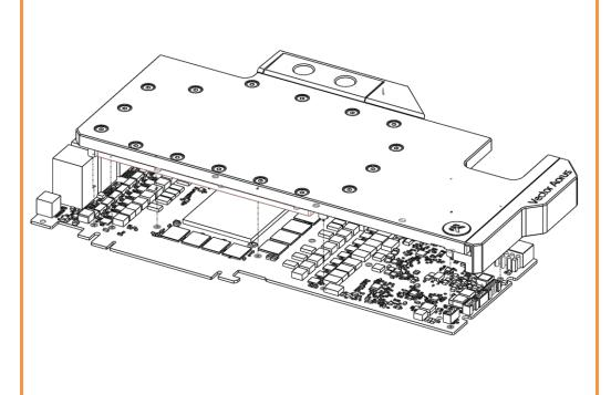
2. ATTACHING THE BLOCK TO THE GRAPHIC CARD. Use a Philips screwdriver screw with the enclosed M2,5x4 AX1 (8) screws and m2,5x6 AX1(6). EKWB recommends users to start tightening the screws around the GPU core and continue outwards. <u>Always use</u> a plastic washer under each and every screw! If the washer is already present on the circuit board (usually around the four GPU core screw holes) there is no need for additional washer.
