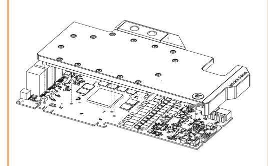
2. ATTACHING THE BLOCK TO THE GRAPHIC CARD. Use a Philips screwdriver screw with the enclosed **M2,5x4 AX1 (12)** screws. EKWB recommends users to start tightening the screws around the GPU core and continue outwards. <u>Always use</u> a plastic washer under each and every screw!
