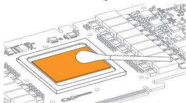
3. CUTTING THERMAL PADS: Your block comes with thermal pads, some of which are already precut. Others have to be cut to smaller chunks in order to cover all the VRM components such as MOSFETs and drivers. PLEASE REMOVE THE PROTECTIVE FOIL FROM BOTH SIDES OF THE THERMAL PADS PRIOR TO INSTALLATION.
