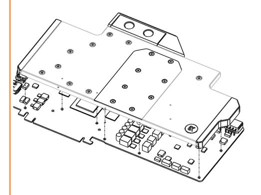
2. ATTACHING THE BLOCK TO THE GRAPHIC CARD. Use a Philips screwdriver screw with the enclosed M2,5x4 AX1 (14) screws. EKWB recommends users to start tightening the screws around the GPU core and continue outwards. <u>Always use</u> a plastic washer under each and every screw! If the washer is already present on the circuit board (usually around the four GPU core screw holes) there is no need for additional washer.
