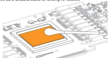
2. APPLYING THERMAL COMPOUND: Wipe off the remains (by using non–abrasive cloth or *q-tip*) of the original thermal compound until the components and circuit board are completely clean. Apply thermal compound: lightly coat *NVIDIA* GPU chip with enclosed EK-TIM Ectotherm thermal grease. EKWB recommends to apply thermal grease in cross form for best performance (see sample picture).
