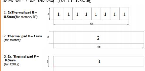
4. PLACING THERMAL PADS ON PCB. Place thermal pads on the circuit board as shown on the picture below. Refer to numbering in previous picture when applying thermal pads of different sizes or thicknesses. EK made sure to provide customers with more than adequate quantity of thermal pads to complete this step.
