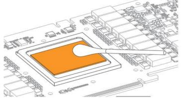
2. APPLYING THERMAL COMPOUND: Wipe off the remains (by using non–abrasive cloth or *q-tip*) of the original thermal compound until the components and circuit board are completely clean. Apply thermal compound: lightly coat *NVIDIA* GPU chip with enclosed EK-TIM Ectotherm thermal grease. EKWB recommends to apply thermal grease in cross form for best performance (see sample picture).
