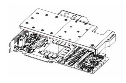
2. ATTACHING THE BLOCK TO THE GRAPHIC CARD. Use a Philips screwdriver screw with the enclosed M2,5x4 AX1 (12) screws. EKWB recommends users to start tightening the screws around the GPU core and continue outwards. <u>Always use</u> a plastic washer under each and every screw! If the washer is already present on the circuit board (usually around the four GPU core screw holes) there is no need for additional washer.
