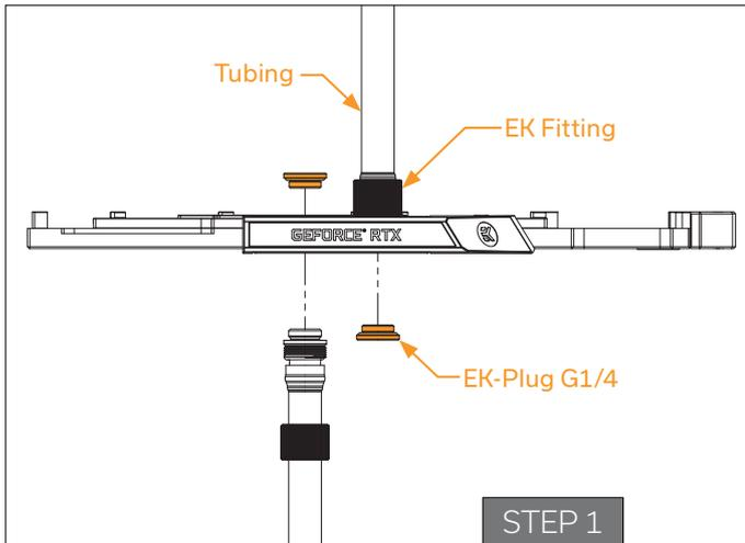
Screw in the two G1/4 threaded male fittings. Attach the liquid cooling tubes and connect the water-block(s) into the cooling circuit. **EKWB recommends using EK fittings with the EK-Vector series water blocks.** To ensure that the tubes are securely attached to the barb/fittings, please use hose clamps or an appropriate substitute.
