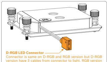
have 4 cables. If you connect D-RGB led to ordinary RGB header you will damage your motherboard or LED strip.
