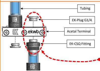
Screw in the two G1/4 threaded male fittings. Attach the liquid cooling tubes and connect the water-block(s) into the cooling circuit. **EKWB recommends using EK-ACF fittings with the EK-FC water blocks**. To ensure that the tubes are securely attached to the barb/fittings, please use hose clamps or an appropriate substitute.
