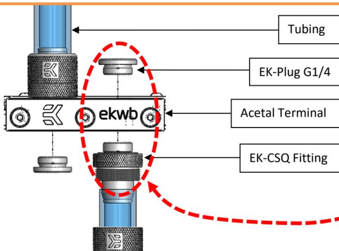
Screw in the two G1/4 threaded male fittings. Attach the liquid cooling tubes and connect the water-block(s) into the cooling circuit. **EKWB recommends using EK-ACF fittings with the EK-FC water blocks.** To ensure that the tubes are securely attached to the barb/fittings, please use hose clamps or an appropriate substitute.
