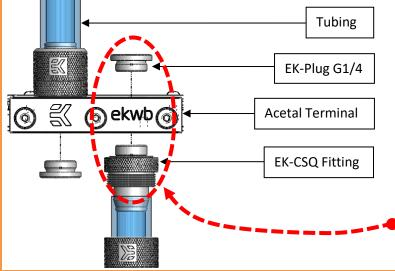
Screw in the two G1/4 threaded male fittings. Attach the liquid cooling tubes and connect the water-block(s) into the cooling circuit. **EKWB recommends using EK-ACF fittings with the EK-FC water blocks**. To ensure that the tubes are securely attached to the barb/fittings, please use hose clamps or an appropriate substitute.
