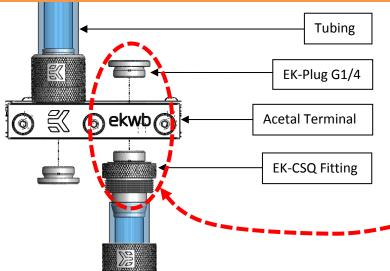
Screw in the two G1/4 threaded male fittings. Attach the liquid cooling tubes and connect the water-block(s) into the cooling circuit. **EKWB recommends using EK-CSQ fittings with the EK-FC R9-290X series water blocks**. To ensure that the tubes are securely attached to the barb/fittings, please use hose clamps or an appropriate substitute.
